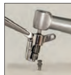
3. Push collar out by rotating the screw
