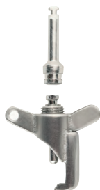
Collar extractor for angle piece
