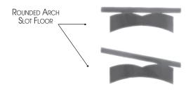
Synergy®'s rounded arch slot floor reduces friction since the arch wire contacts the floor at only two points.
